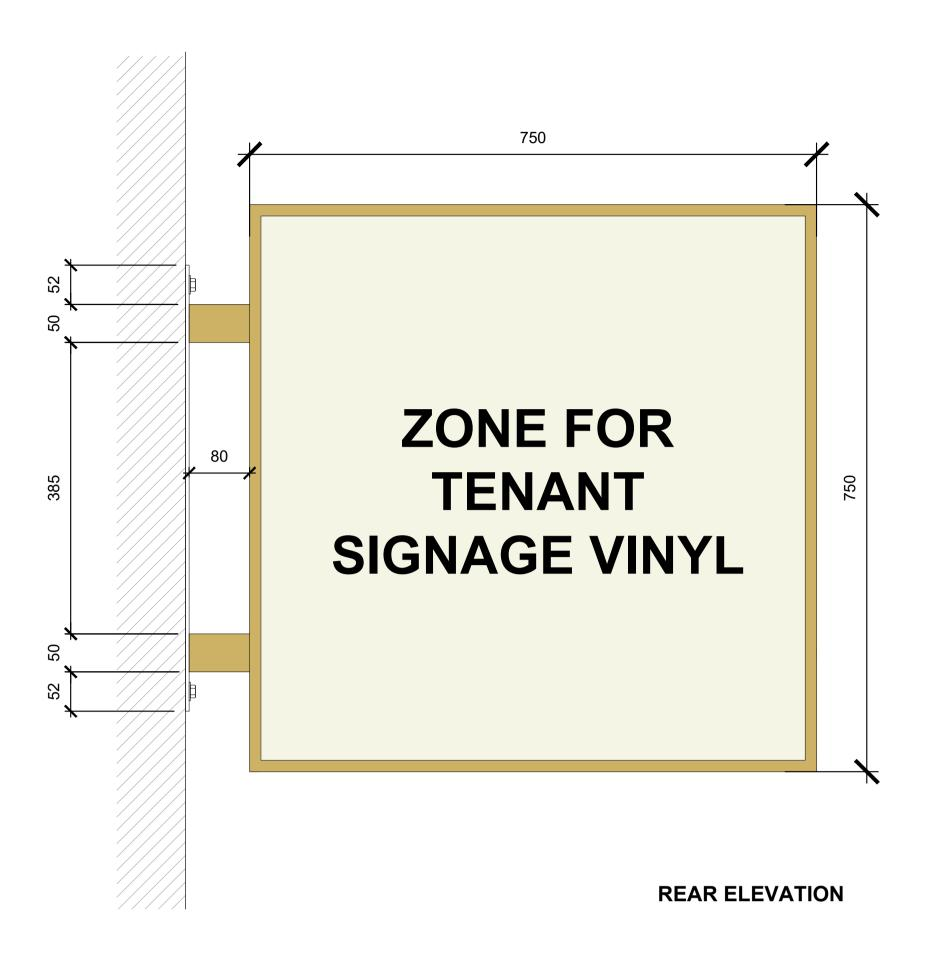
Sign comprising 750mm x 750mm aluminium sign carcass with 2N° ← 50x50mm aluminium box section arms welded to internal vertical plates within carcass and 450x125x5mm thick aluminium wall plate, all finished powder coated Bronze RAL Colour to match existing curtain wall externally.
