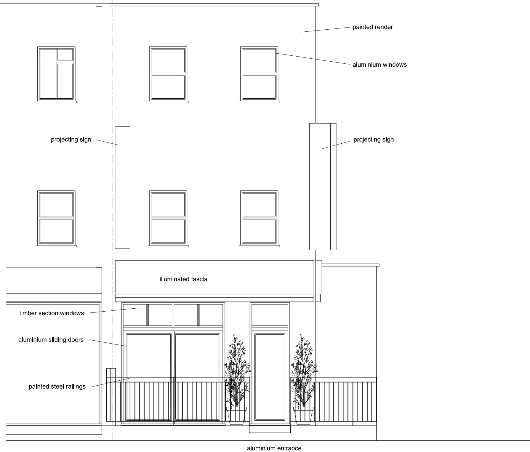
Existing Front Elevation
