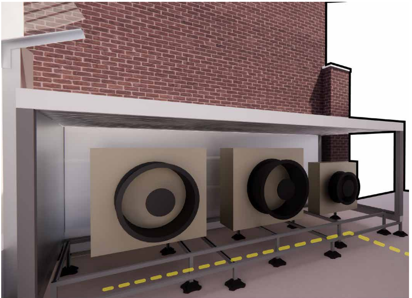
Fig. 16: Visual of the access yard and the placement of the condensers. The dashed yellow line denotes the path of the pipework beneath the paving.
