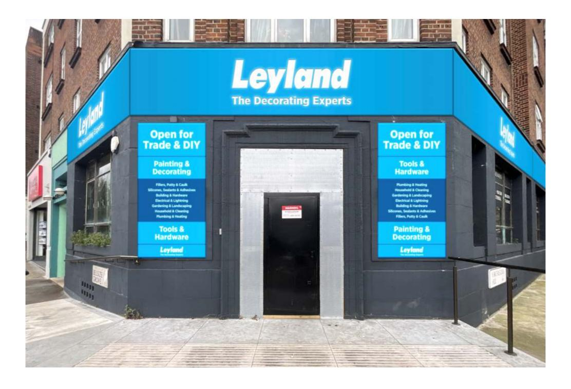
1100mm (W) x 2000mm (H) 3mm aluminium trays powder coated Blue RAL5015 with opal acrylic faces with a vinyl graphic applied. Internally illuminated via Cool White LEDS. 2no. required – 1 either side of door.
