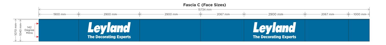
3mm aluminium folded fascia 100mm deep coated blue RAL 5015 with fret cut and opal backed text, internally illuminated via cool white LEDs & power supplies to suit.
