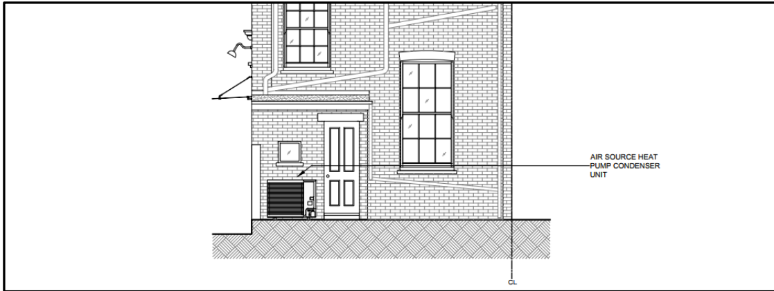
Figure 2.3 Plant location positions (Image Source: Schneider Designers)
