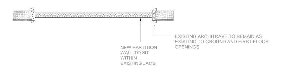
GROUND AND FIRST FLOOR DOUBLE DOOR OPENING TYPICAL PLAN 1:20
