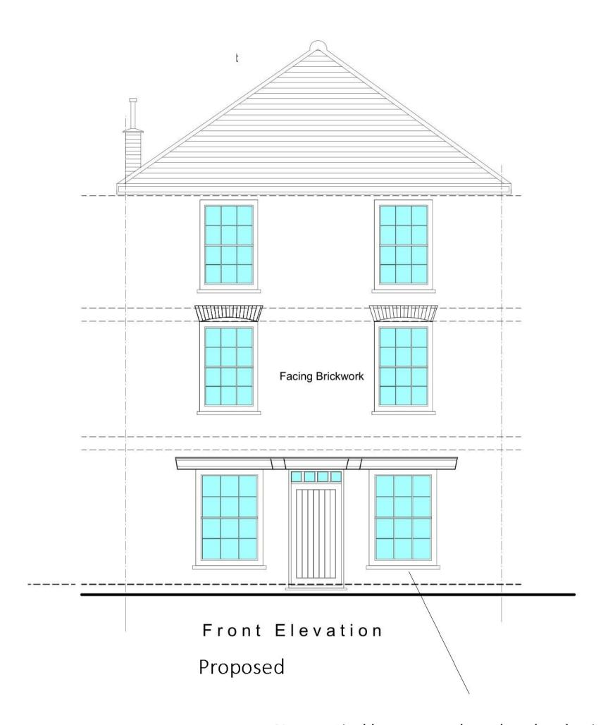
New vertical hung secondary glazed sash window by Selectaglaze, Series 90VS counterbalanced vertical slider comprising two sash windows, each single glazed with 7.5mm laminated clear glass. Frame powder painted white RAL 9910, fitted into existing reveal, recessed minimum 140mm behind existing wooden sash window. Sash rails centred to match existing fenestration.
