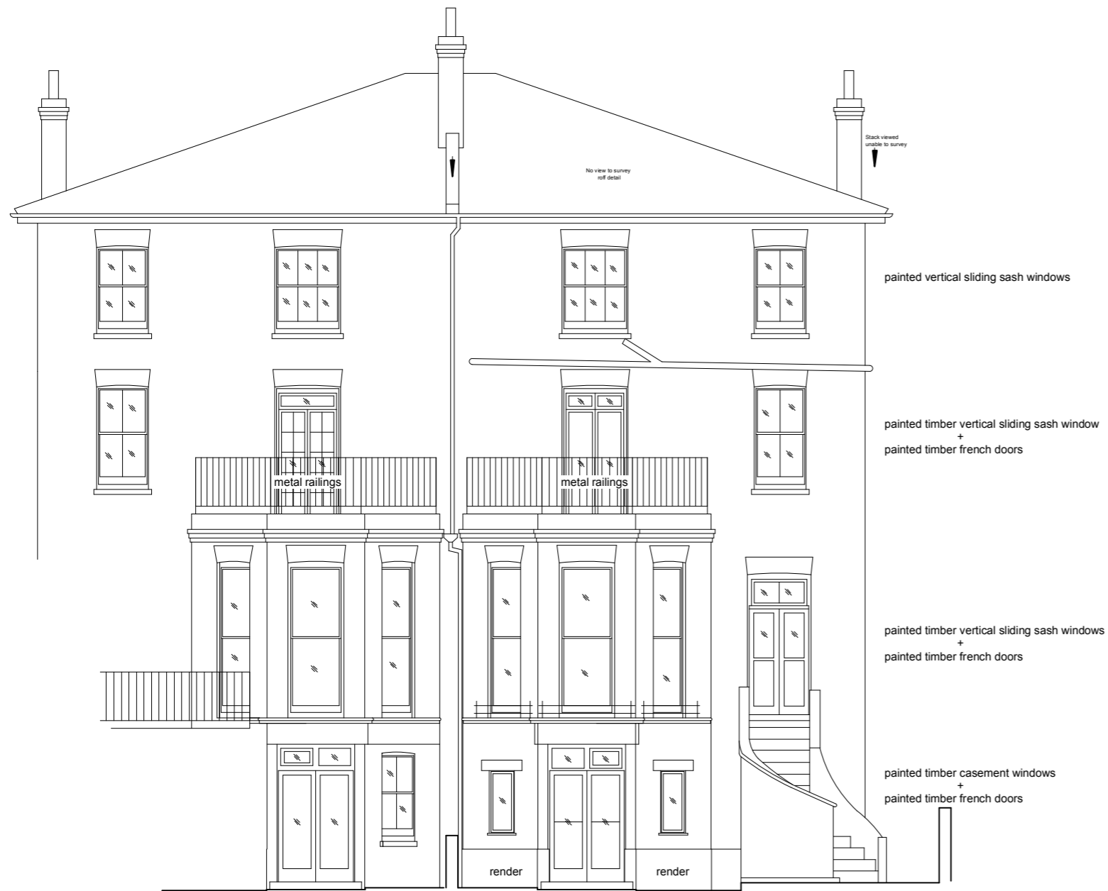
Existing Rear Elevation
