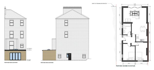
The proposed rear extension has been designed to be proportionate and subordinate to the application property. From the original rear wall, the extension has a modest depth of 3.8 metres, which matches the existing neighbouring rear extension at no. 96 Agar Grove. The proposed rear extension has a moderate maximum height of 3.28 metres.
