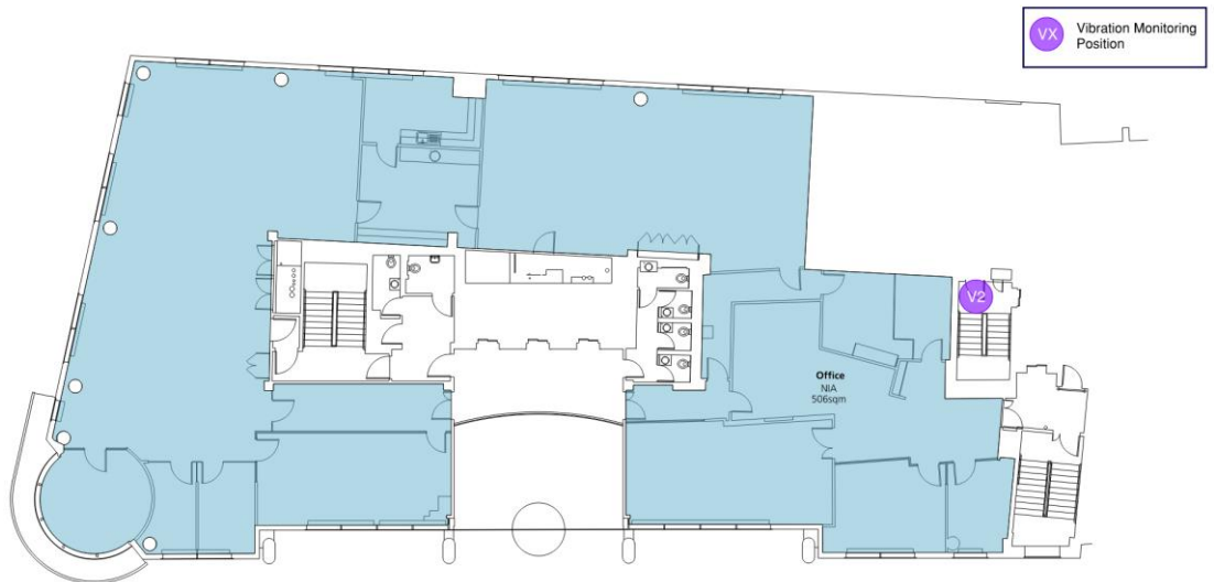
Figure 4.5: First Floor Plan Showing Vibration Monitoring Locations
