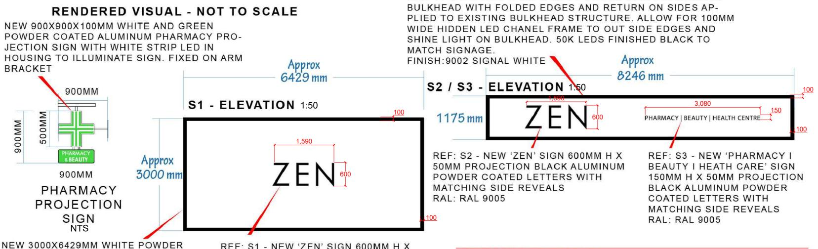
NEW 3000X6429MM WHITE POWDER COATED ALUMINUM BULKHEAD WITH FOLDED EDGES AND RETURN ON SIDES APPLIED TO EXISTING BULKHEAD STRUCTURE. ALLOW FOR 100MM WIDE HIDDEN LED CHANEL FRAME TO OUT SIDE EDGES AND SHINE LIGHT ON BULKHEAD. 50K LEDS FINISHED BLACK TO MATCH SIGNAGE. FINISH:9002 SIGNAL WHITE
