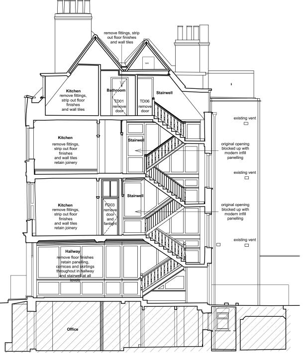
01 Existing Section C 005 1:100@A3; 1:50@A1 02 Existing Section D 005 1:100@A3; 1:50@A1
