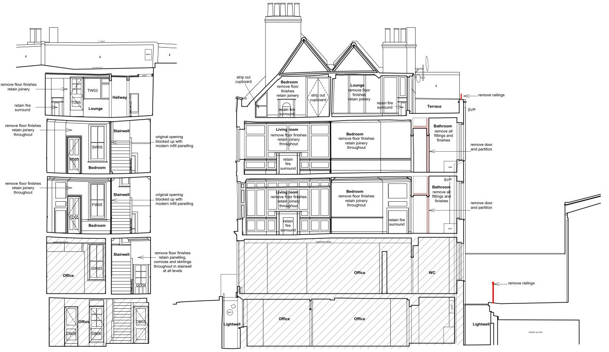
01 Existing Section A 004 1:100@A3; 1:50@A1 02 Existing Section B 004 1:100@A3; 1:50@A1
