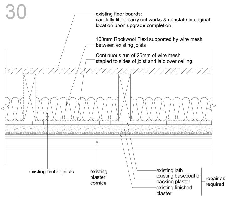
Lath & plaster ceilings are generally accepted as offering about 20 minutes fire integrity untreated. To achieve the full 30FR required the plaster should be treated with Envirograf intumescent coating (1 x coat EP/CP/P primer or 1 x coat Stabond sealer +2 x coats EP/CP intumescent + 1 x coat HW AEC acrylic emulsion protective topcoat).
