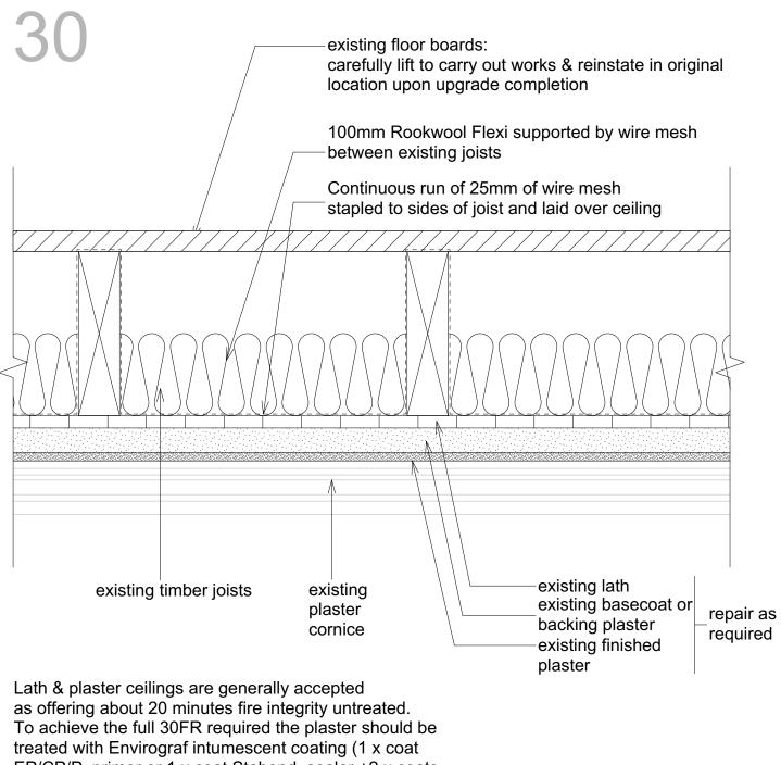
treated with Envirograf intumescent coating (1 x coat EP/CP/P primer or 1 x coat Stabond sealer +2 x coats EP/CP intumescent + 1 x coat HW AEC acrylic emulsion protective topcoat).
