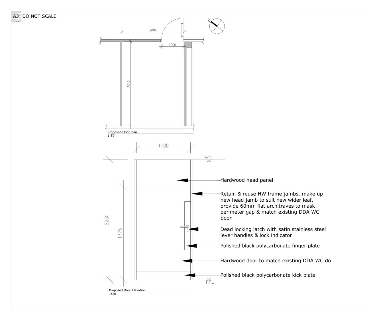
ALL DIMENSIONS, LEVELS AND CLEARANCES TO BE CHECKED ON SITE PRIOR TO WORKS COMMENCING
