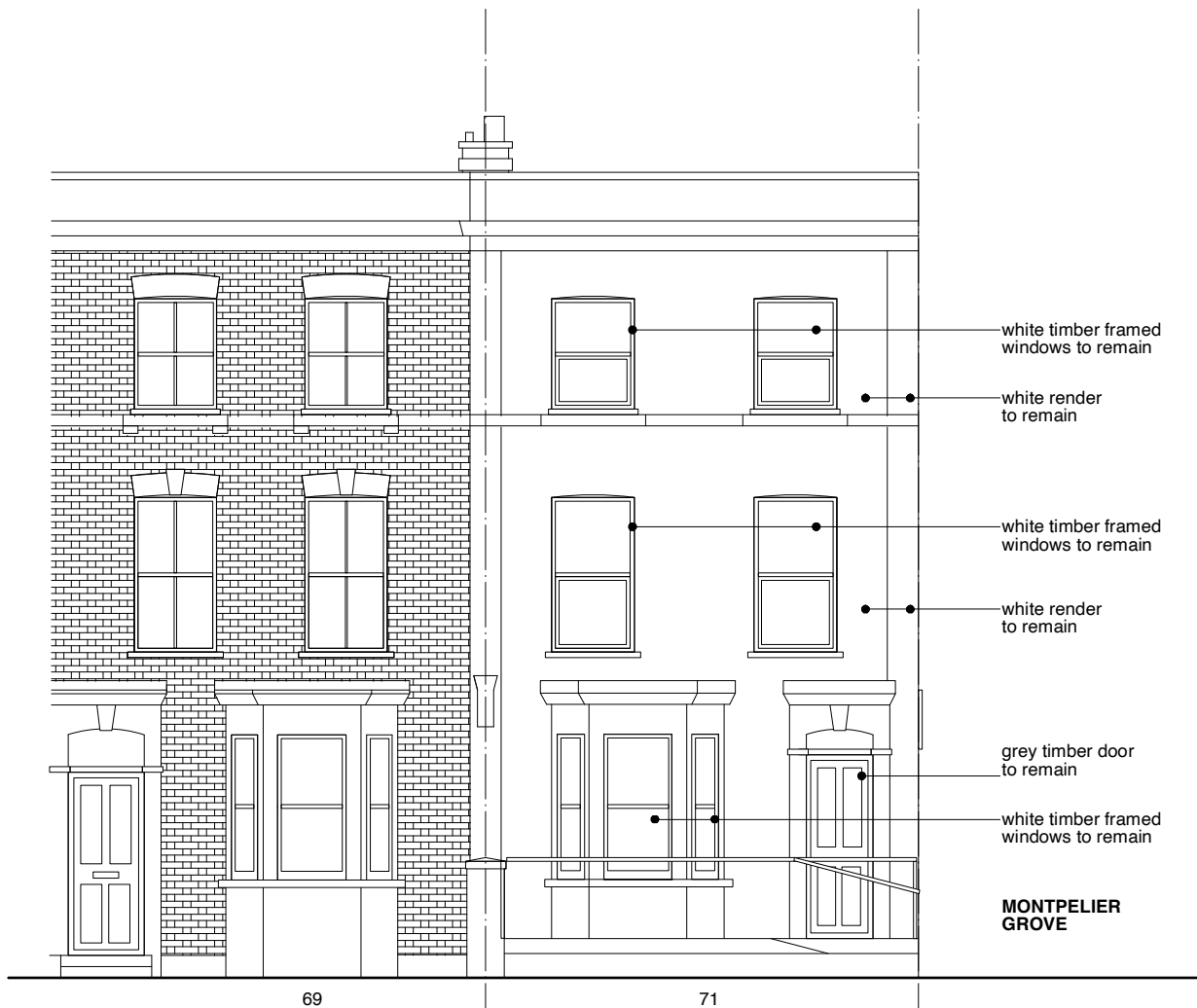
PROPOSED FRONT ELEVATION (to remain as existing)
