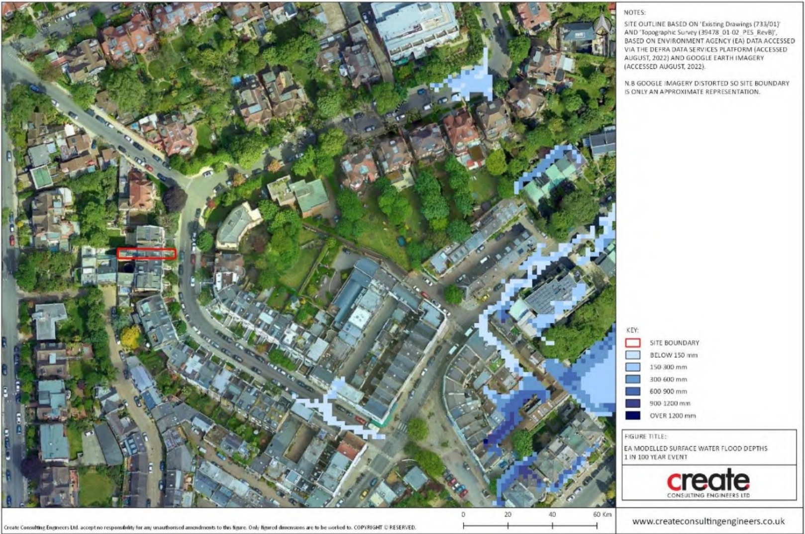
Figure 5: EA Surface Water Depth (Medium Risk Event) Source: Defra Data Services Platform ( https://environment.data.gov.uk/ )
