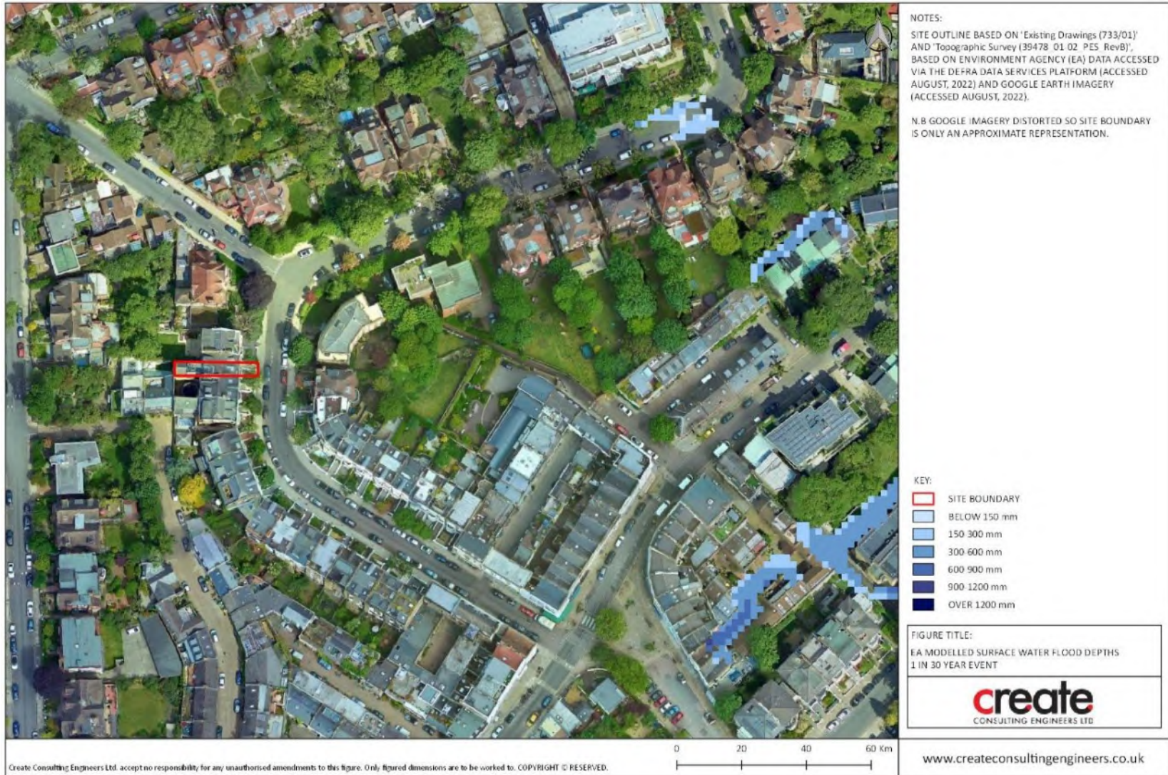
Figure 4: EA Surface Water Depth (High Risk Event)
