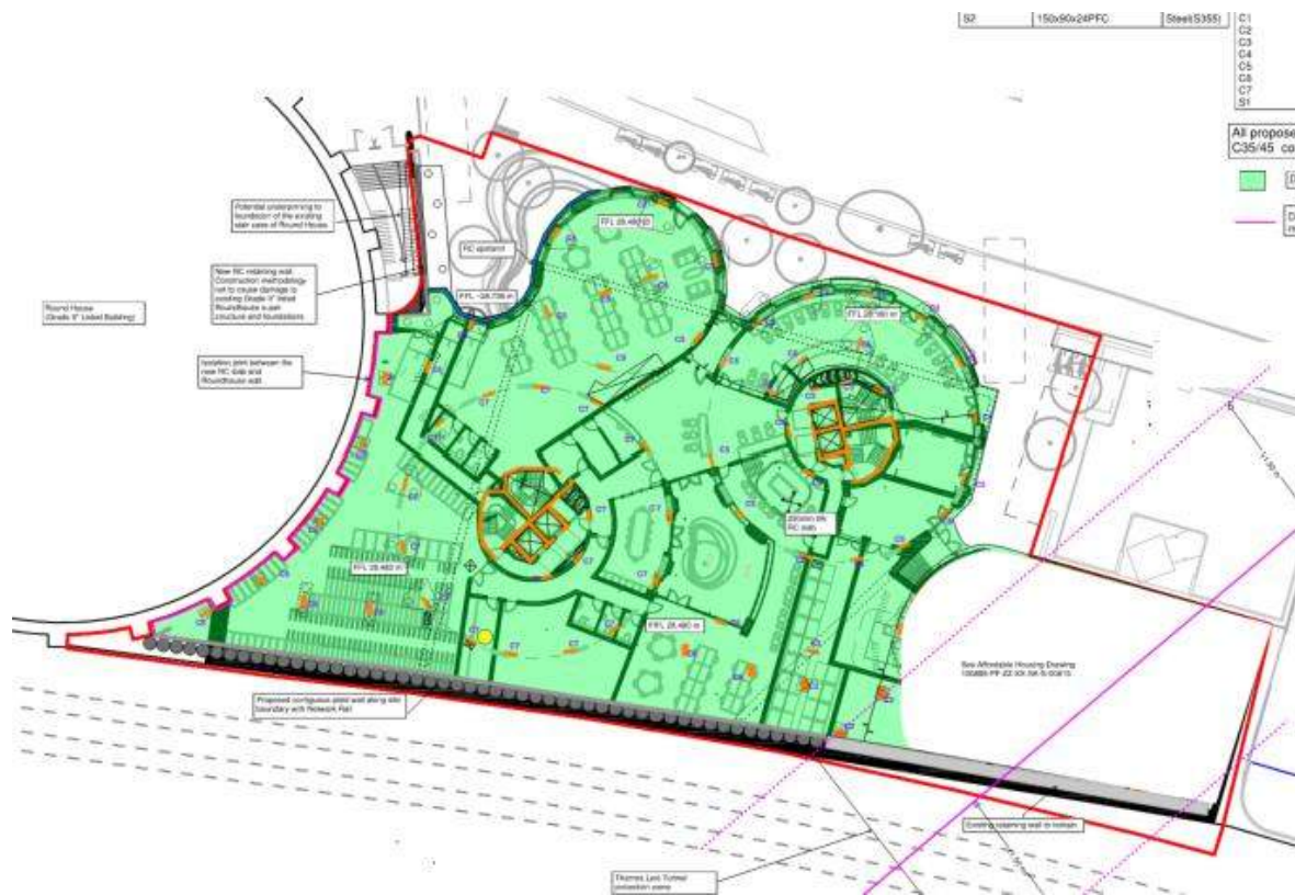
Figure 31 - Proposed ground floor plan showing the extent of the proposed contiguous piled wall.
