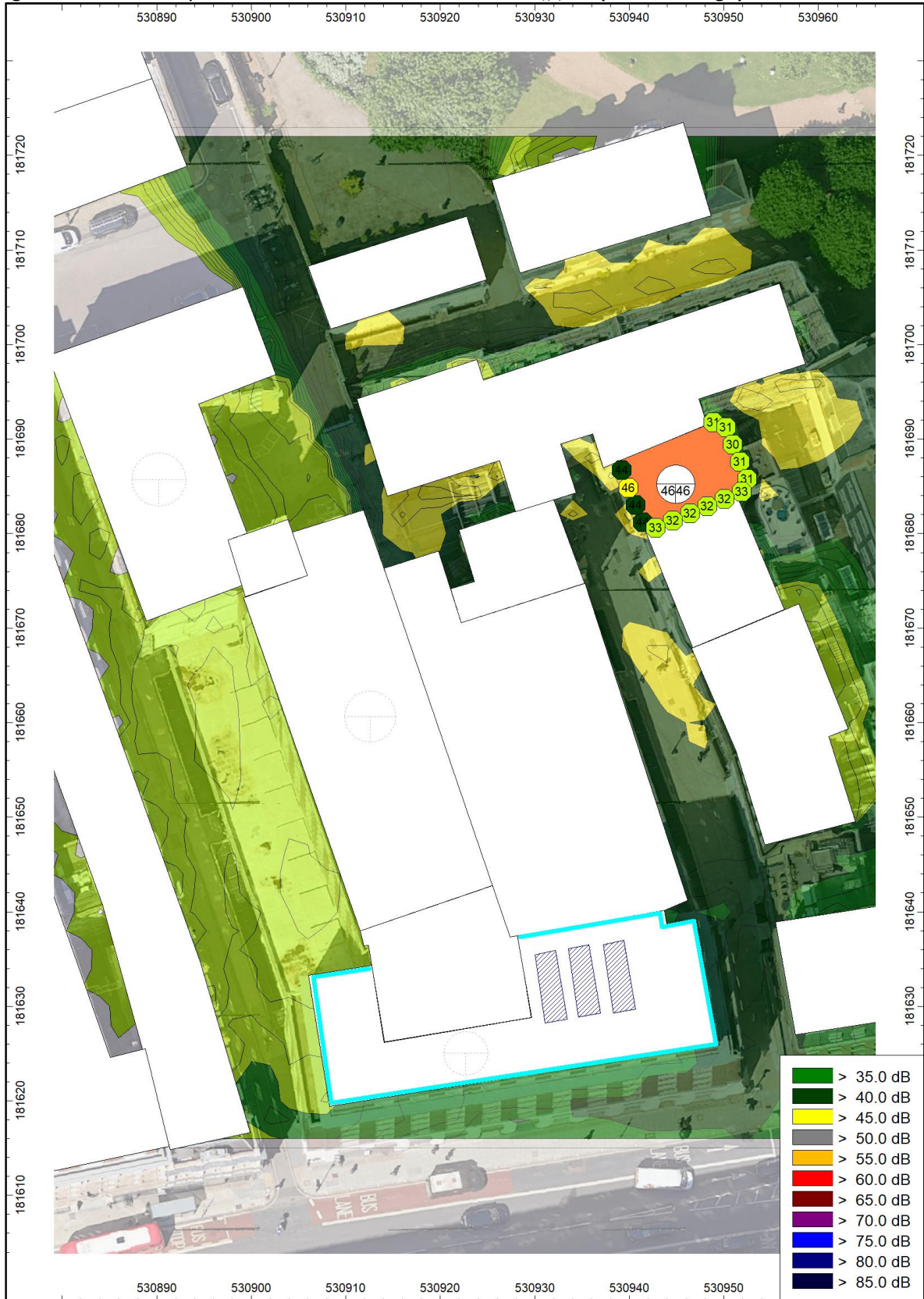
Figure 5: Predicted Specific Sound Level of New chillers L_{Aeq(T)} dB (NSR in orange)
