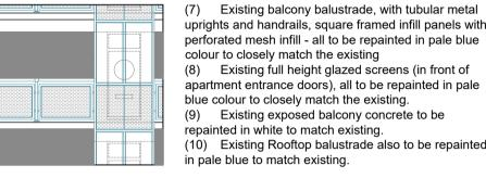
uprights and handrails, square framed infill panels with perforated mesh infill - all to be repainted in pale blue colour to closely match the existing (8) Existing full height glazed screens (in front of apartment entrance doors), all to be repainted in pale blue colour to closely match the existing. (9) Existing exposed balcony concrete to be repainted in white to match existing. (10) Existing Rooftop balustrade also to be repainted in pale blue to match existing.
