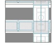
(7) Existing balcony balustrade, with tubular metal uprights and handrails, square framed infill panels with perforated mesh infill, (8) Full height glazed screens (in front of apartment entrance doors), all in pale blue colour. (9) Exposed balcony concrete in white. (10) Rooftop balustrade in pale blue.
