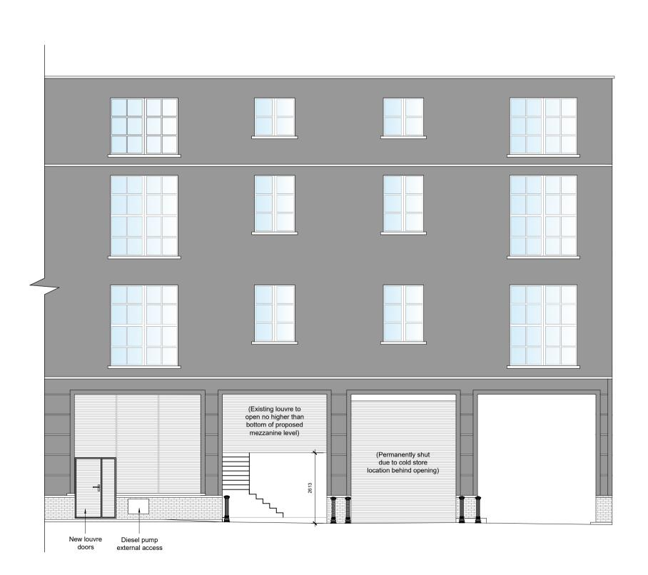
Proposed Rear Elevation (shutters at max opening height) Scale - 1:50@A1
