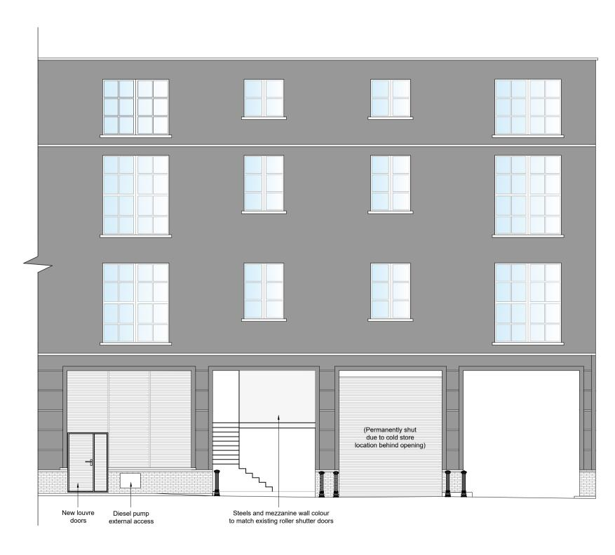
Proposed Rear Elevation (showing mezzanine internally)
