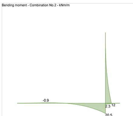
**Check stem design at base of stem**Depth of section  $h = 325$  mm**Rectangular section in flexure - Section 6.1**Design bending moment  $M = 14.9$  kNm/m  $K = 0.007$   $K' = 0.207$  **$K' > K$  - No compression reinforcement is required**Tens.reinforcement required  $A_{sr.req} = 134$  mm<sup>2</sup>/m
