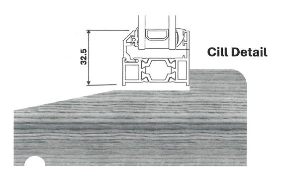
H. Section of new window – manufacturer's diagram showing specification and dimensions of the new window (fixed pane and casement) of the showing (entitled Conservation 39 window into ... timber frame)
