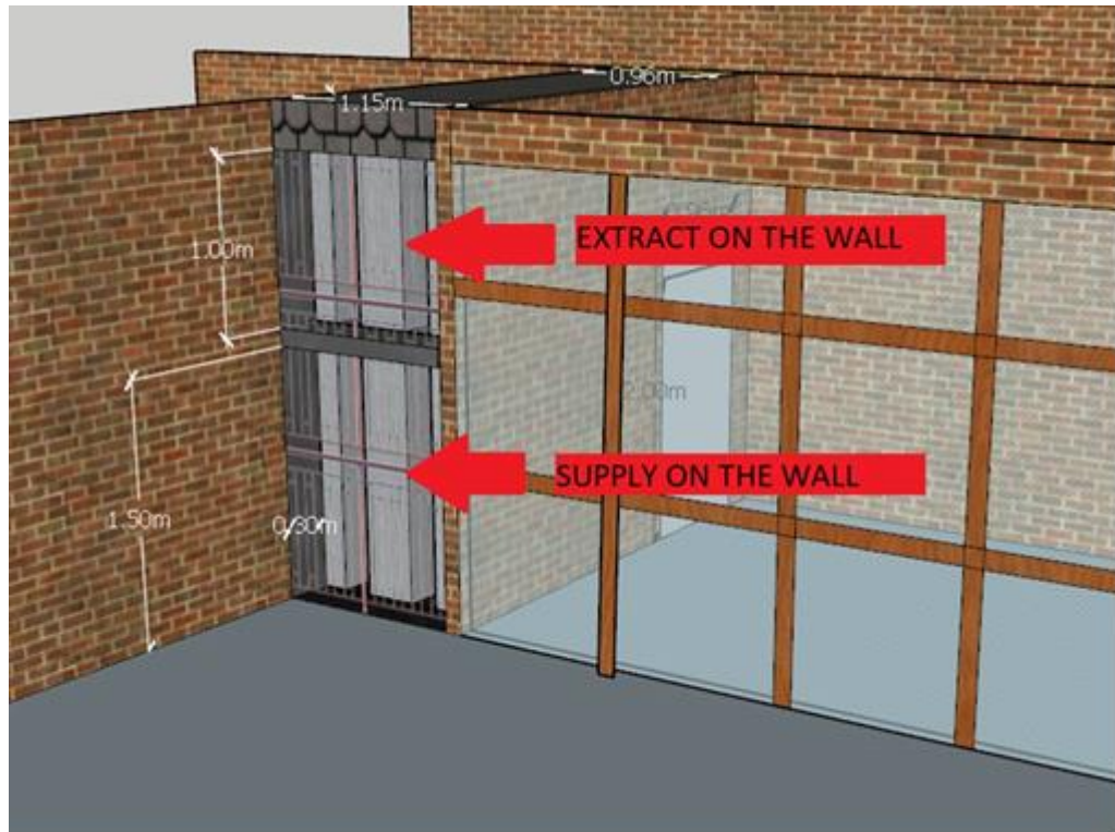
Figure 7: Required enclosure for the ASHP.
