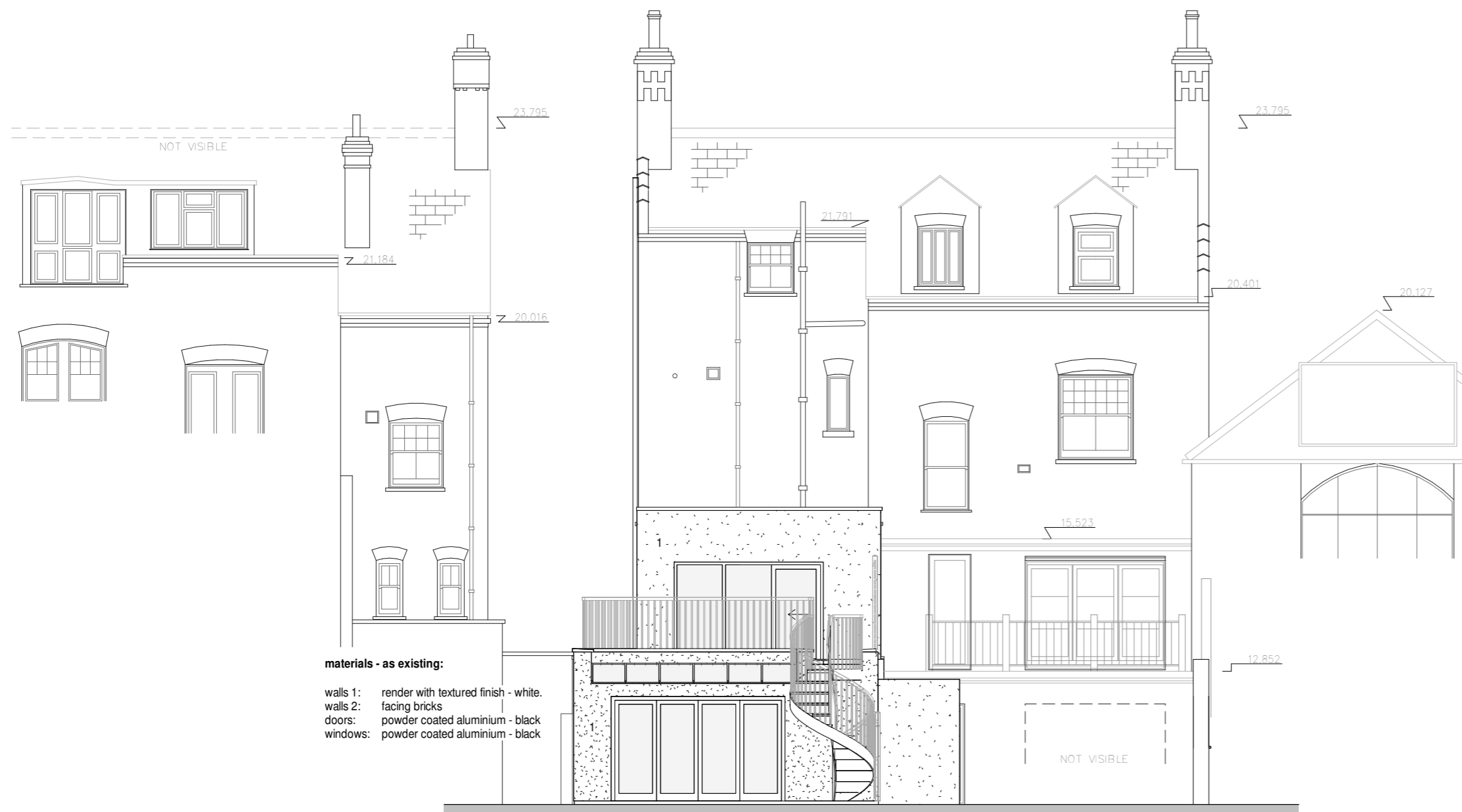
2 07.4 North elevation - side ext - as existing p402 1 : 100
