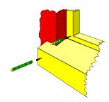
Typical example area identified in sketch: Drill and insert Dry Pins (See Product Sheet).
