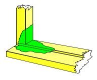
Remove decayed areas back to sound timber using the PROFI with round cutter. Check for moisture content using the WOOD CONDITION METER, apply DRY FIX, allow for penetration and fill with DRY FLEX RP. After curing, sand to shape and apply paint finish. This will give a permanent repair to the areas affected by wood decay, it will be stronger than the original timber and is flexible enough to allow movement without loss of strength or adhesion. See repair method 2.
