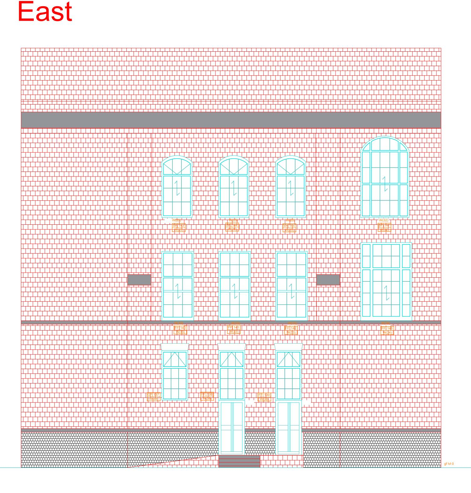
All windows are to be repaired utilising the recognised repair care system and utilising wood species Sapele and Accoya.
