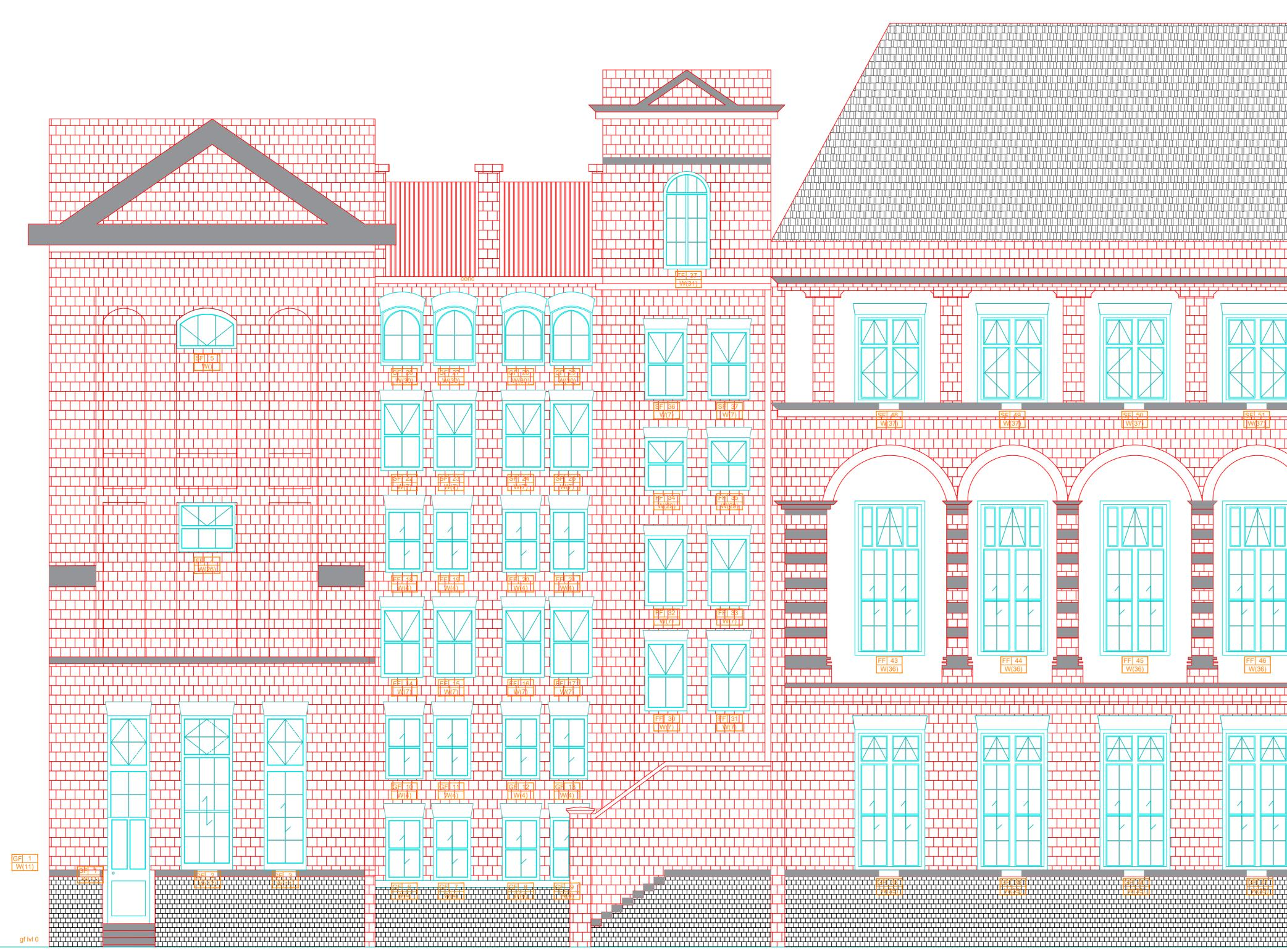
All windows are to be repaired utilising the recognised repair care system and utilising wood species Sapele and Accoya.
