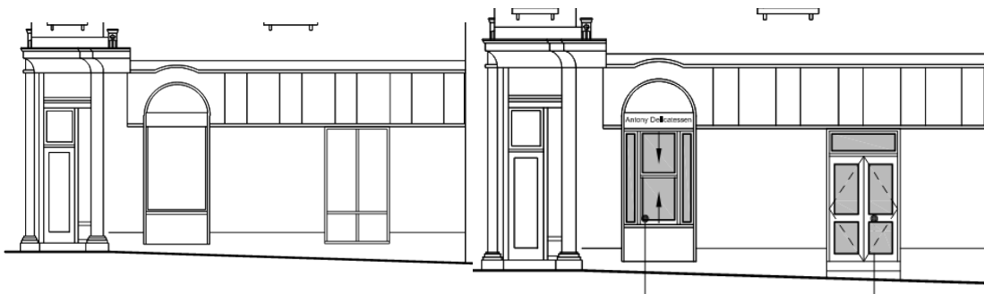
4. Existing side elevation (left) and proposed side elevation (right)
