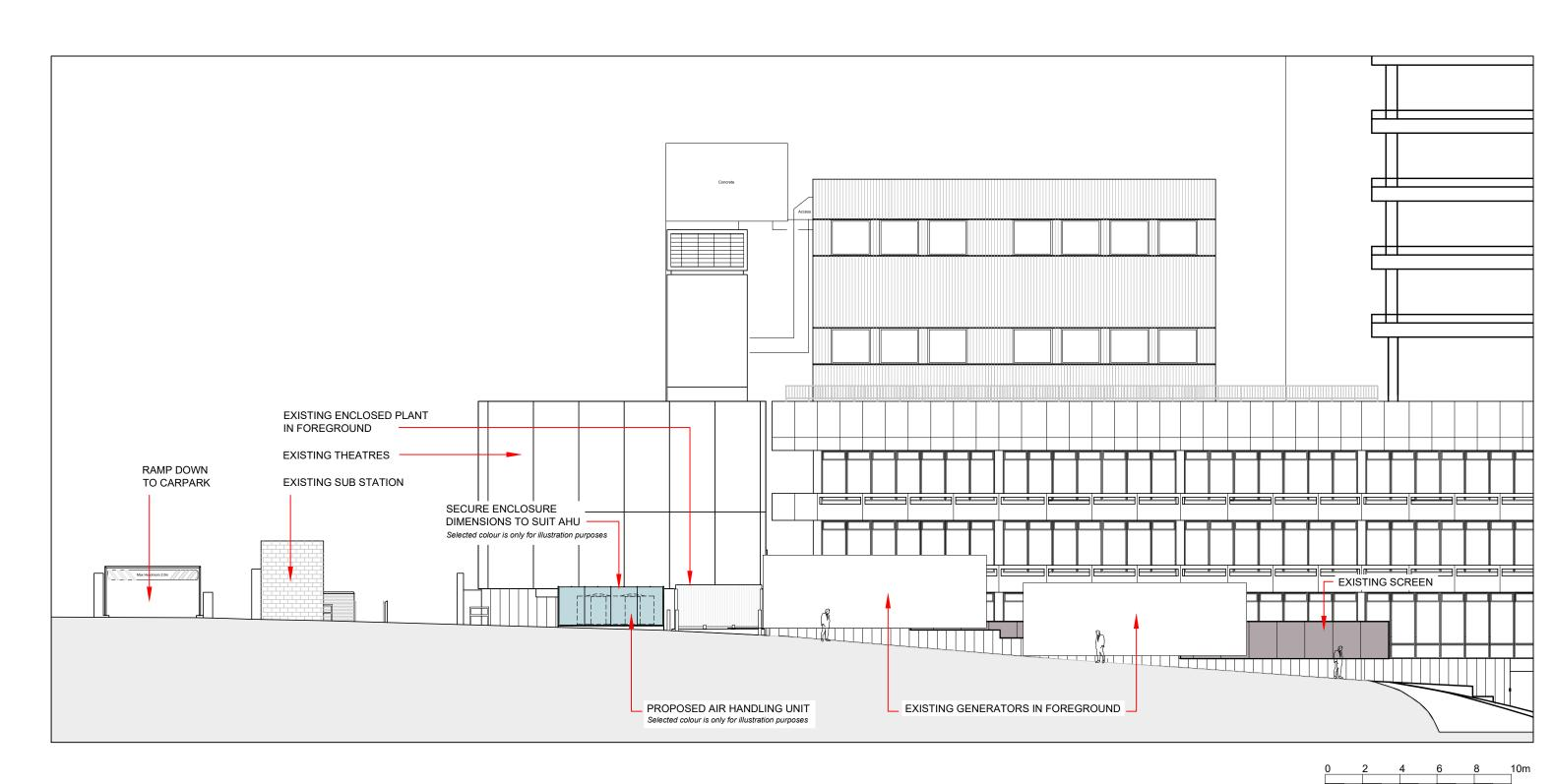
01 Proposed South Elevation (02)002 1:200 @ A3
