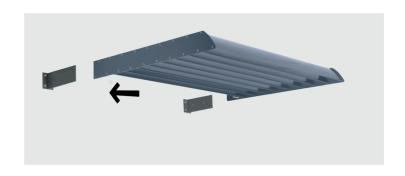
Offer the cassette up inbetween the brackets and loosely fit using the supplied bolts.
