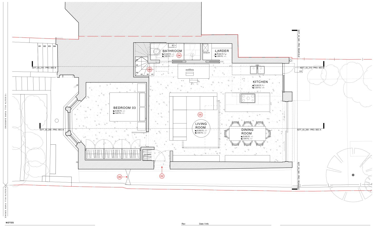
O1 Proposed new double glazed painted timber sash window with profiles to match existing
