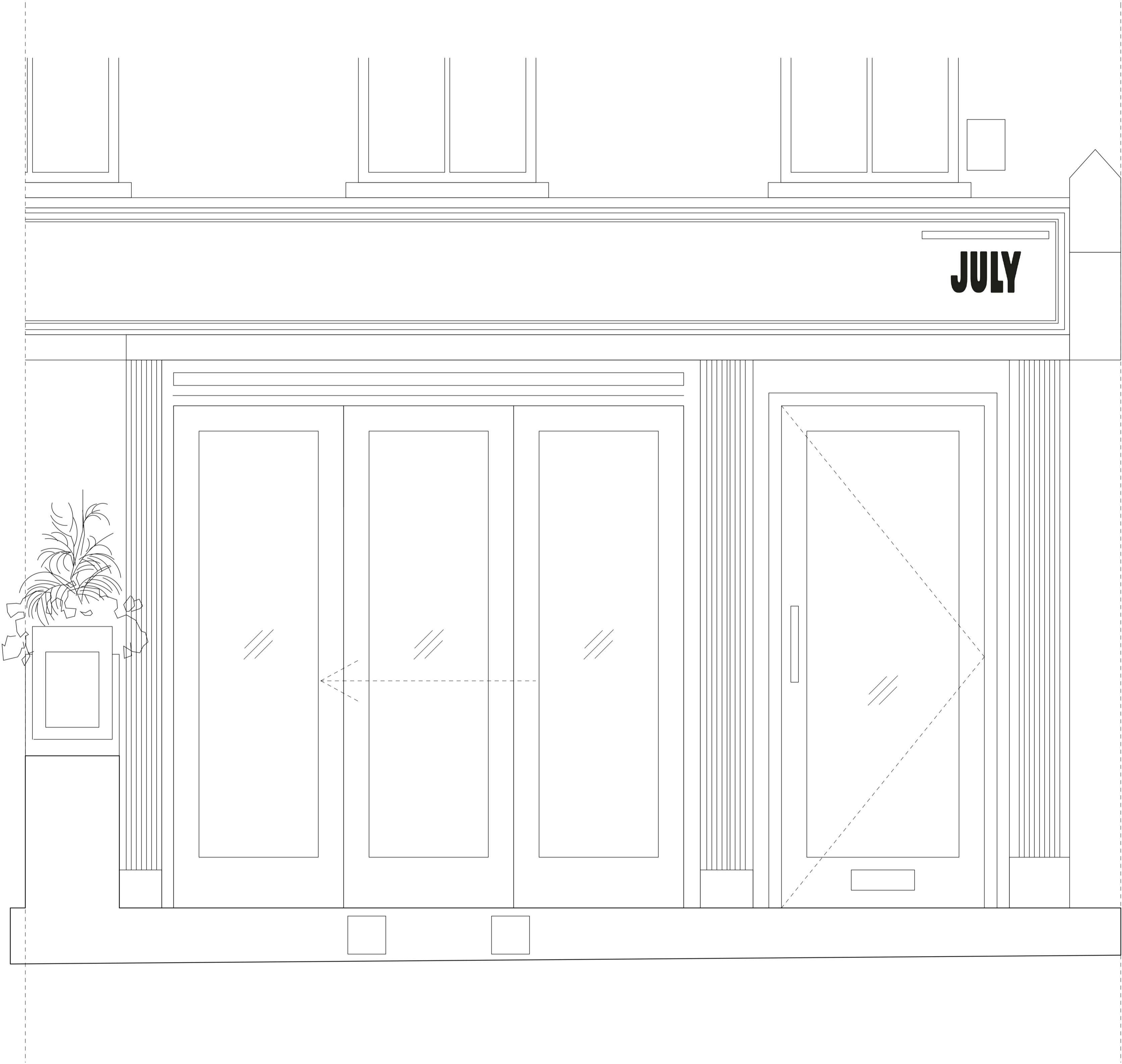
01 FRONT ELEVATION - MINUS AWNING SCALE: 1:10
