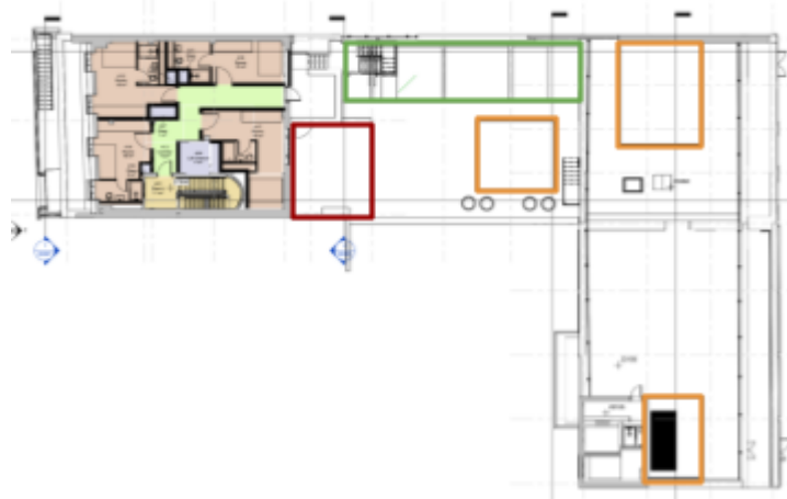
Figure 7: Fourth Floor plan - Courtyard infill (red), Courtyard creation (green), Rooftop plant (orange) - (Source: White Red)
