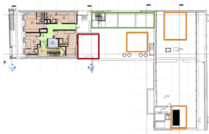
Figure 5: Fourth Floor plan - Courtyard infill (red), Courtyard creation (green), Rooftop plant (orange) - (Source: White Red)
