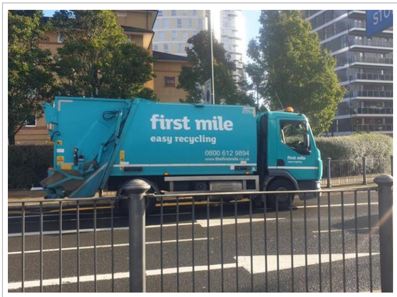
Figure 3.3: Example of 6.7m long refuse collection vehicle.
