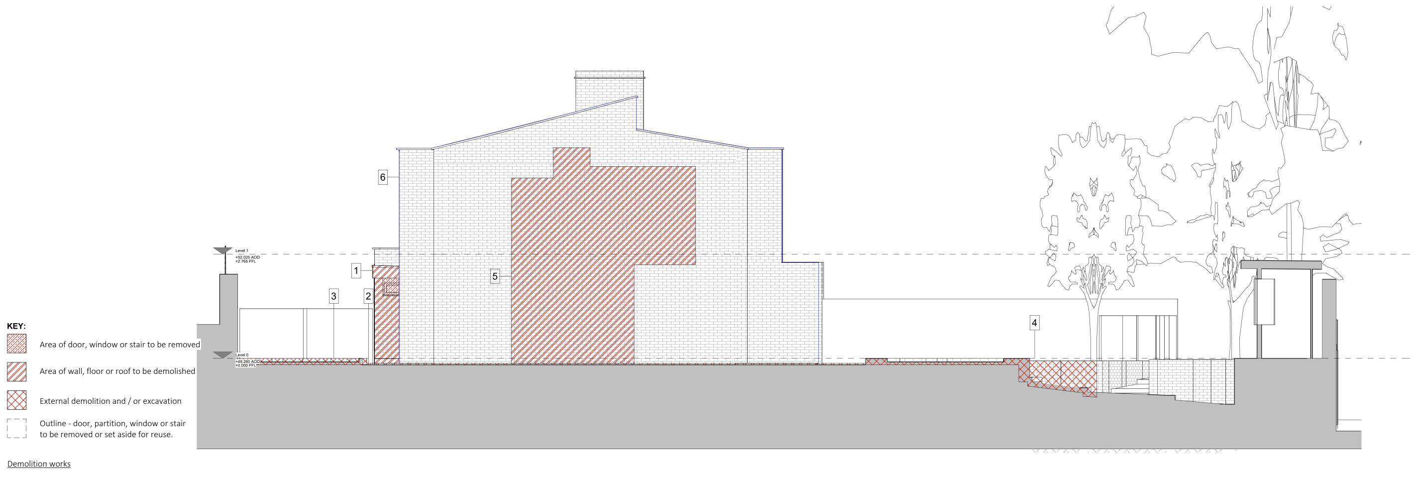
Walls and porch of North West Elevation to be demolished, windows and doors to be removed
