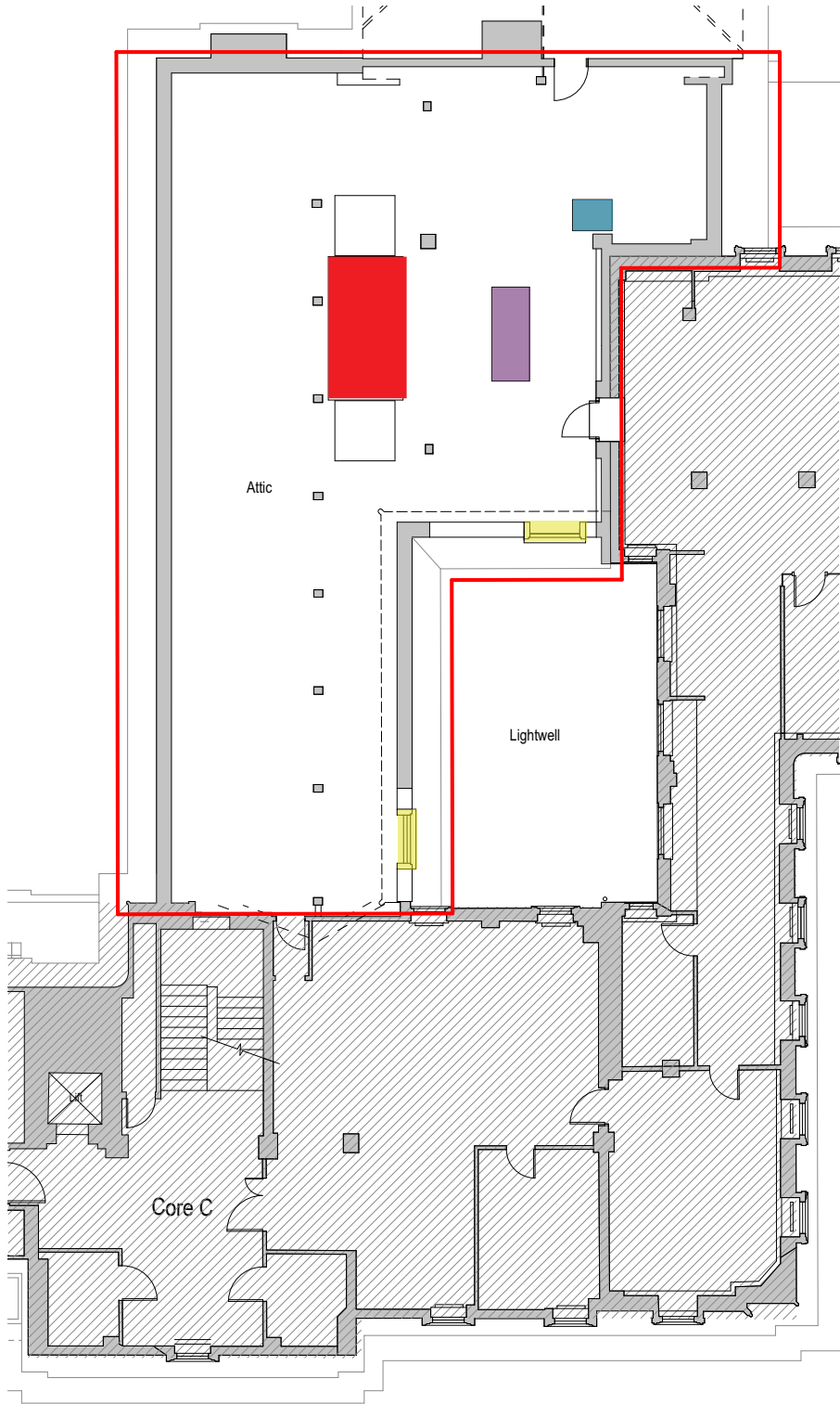
Proposed Level 5 Plan: Showing proposed attic Plant (Water Tanks) in Block F
