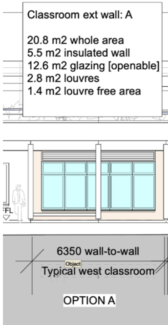
Figure 3 - Window design; openable and maximising daylighting
