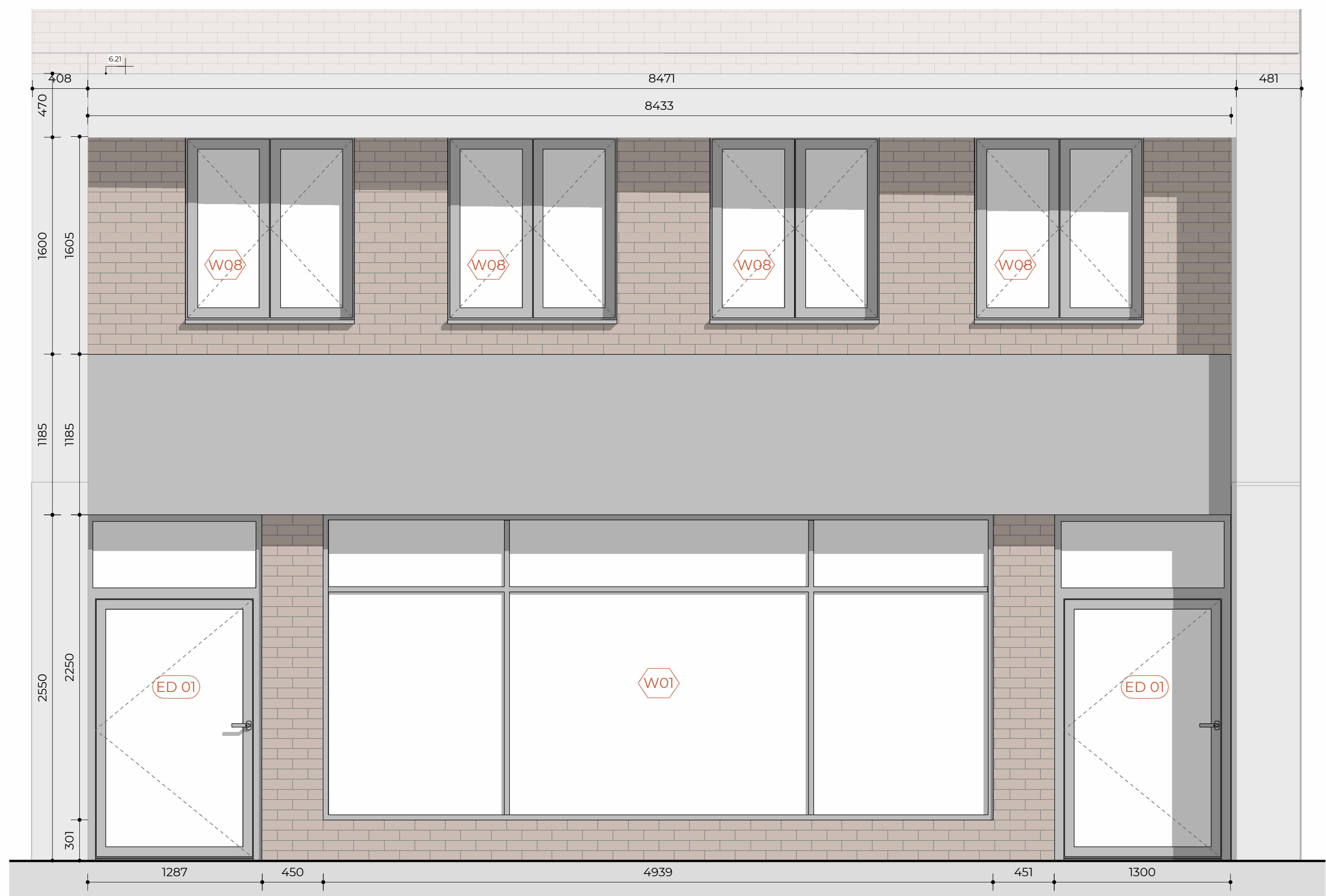
Shopfront Elevation - Scale 1:25
