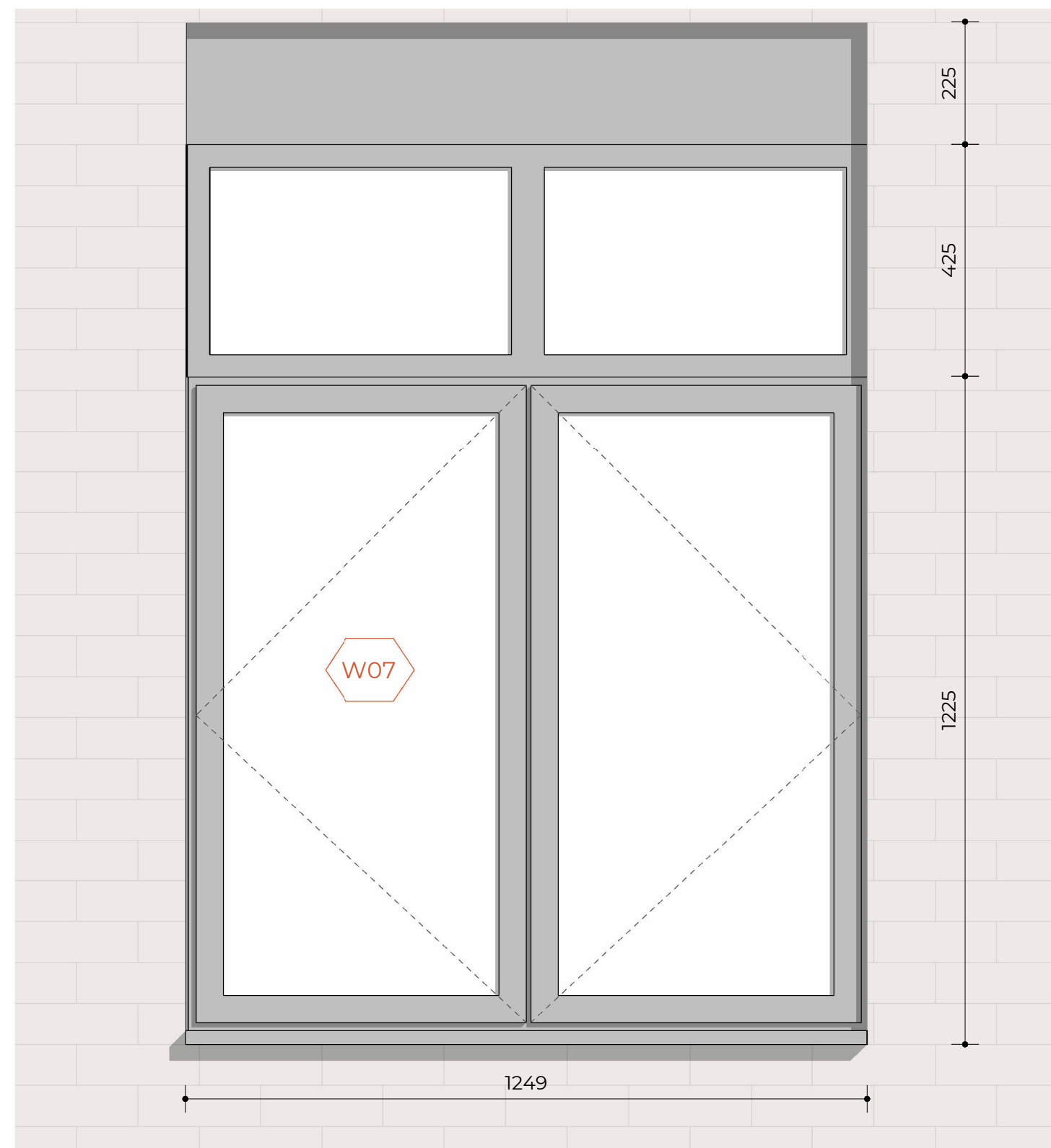
W07 - Front Elevation Second Floor
