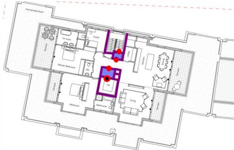
Figure 7 -Block A Ventiladed Lobbies
