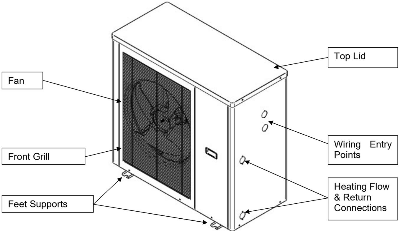
**Figure 2 Typical Construction**
