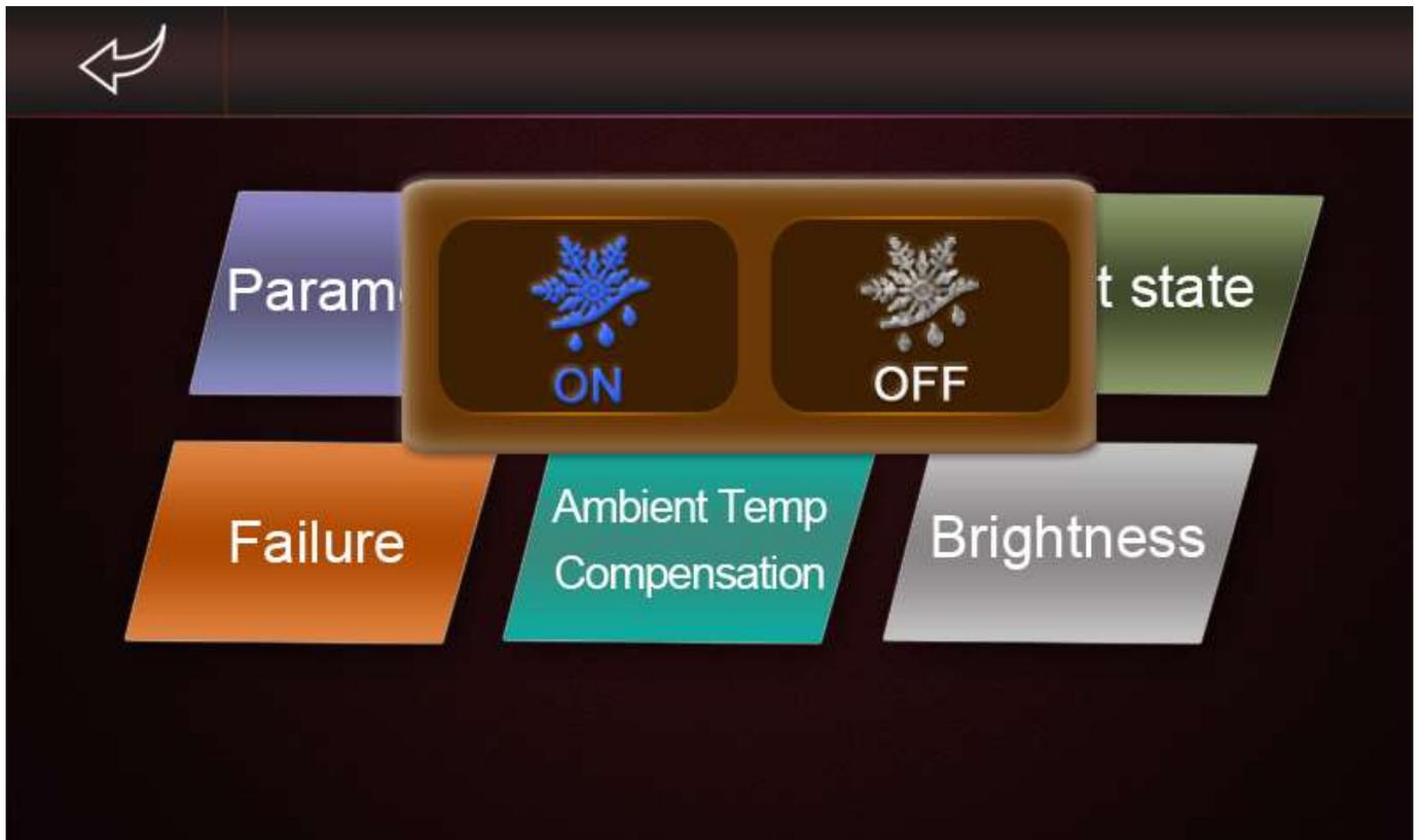
**Unit State** – Press this button to enter the Unit Status Sub-Menu. Pressing the button brings up the following display screen which displays the current status of a number of outputs spread across a number of tabs. These outputs and their functionality are detailed in Table 5 at the end of this chapter:
