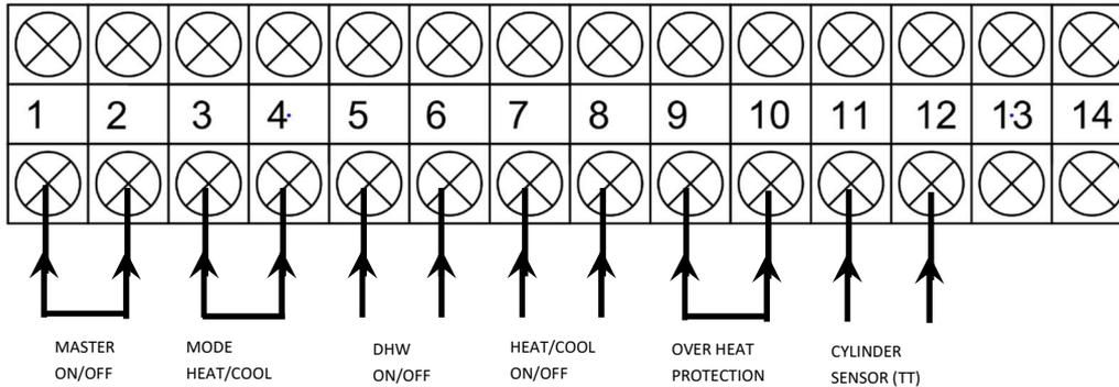
**Figure 31 Installer's Digital Input Connections (AS03)**
