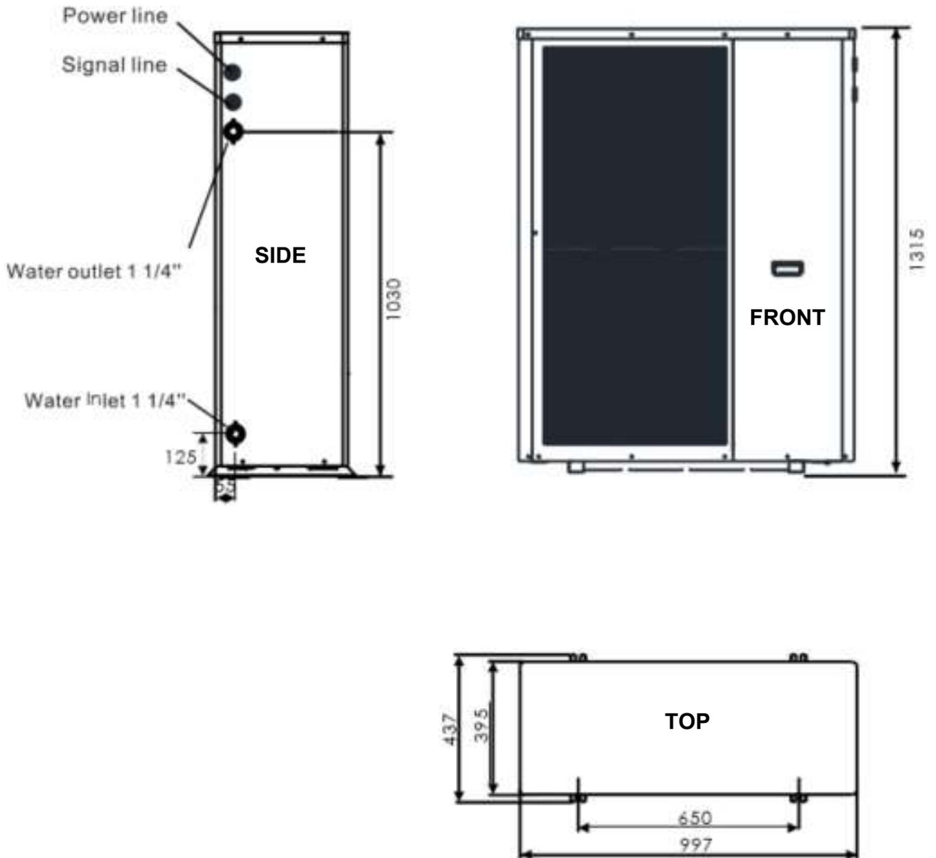
**Figure 25 AS03-R32 Casing Dimensions & Heating Connection Locations**
