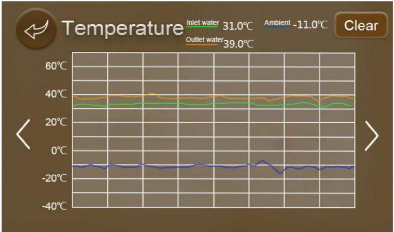
**Figure 22 Heating Flow & Return Temperature Graph Screen**
