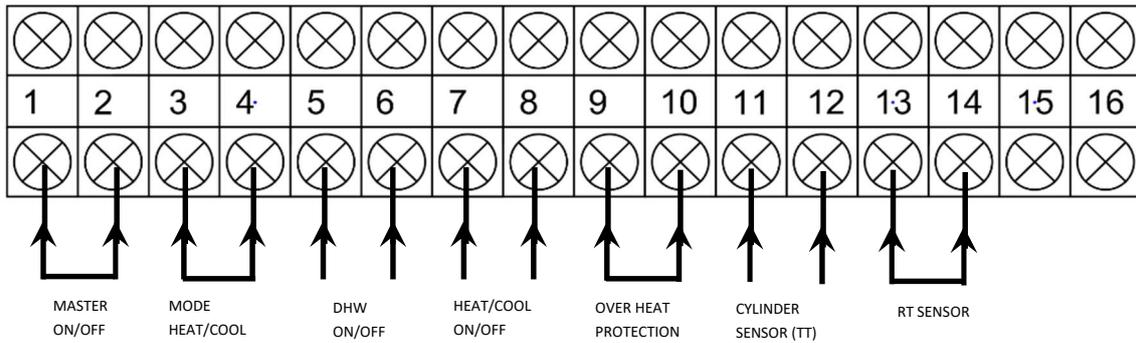
**Figure 30 Installer's Digital Input Connections (AS01 & AS02)**
