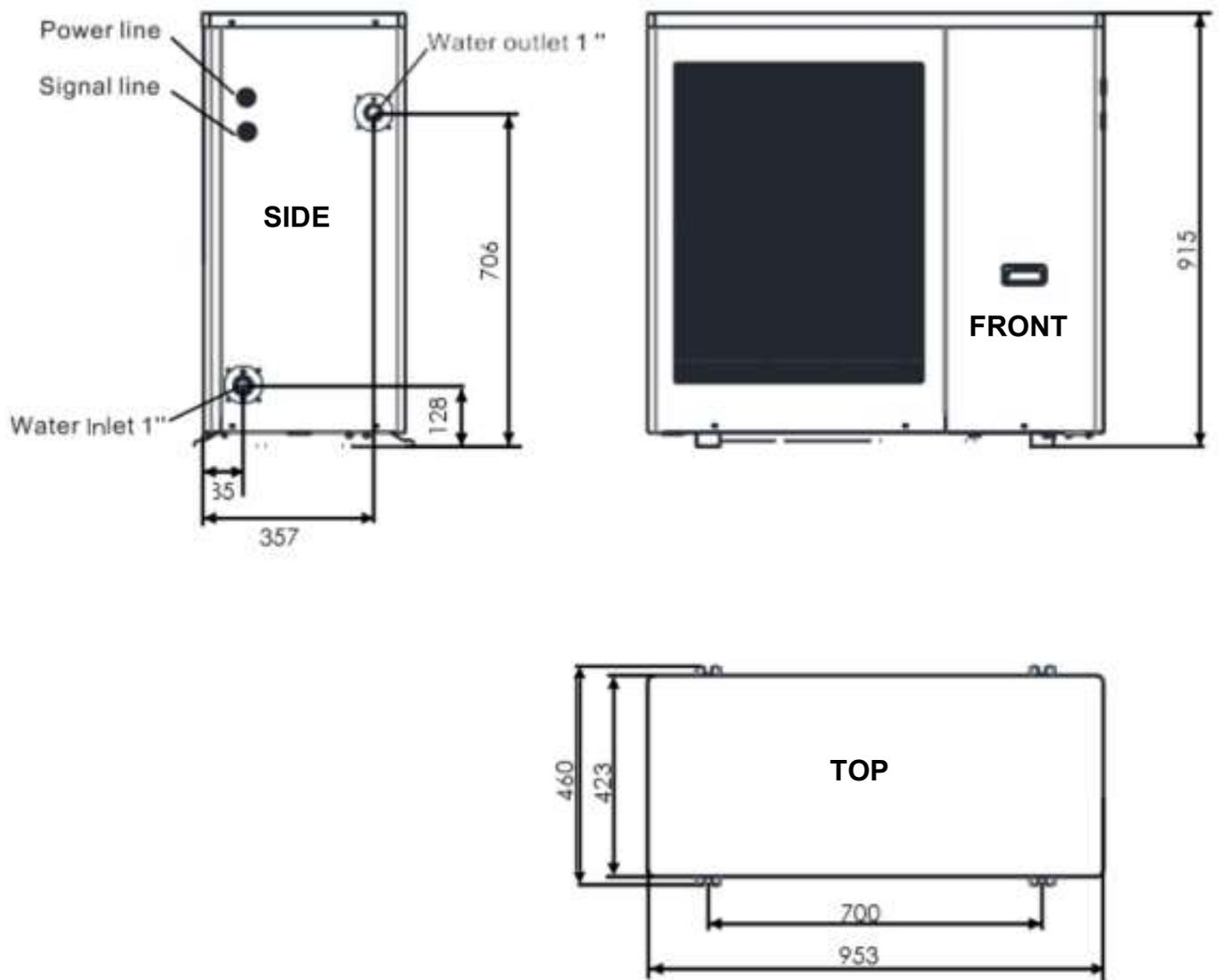
Figure 24 AS02-R32 Casing Dimensions & Heating Connection Locations
