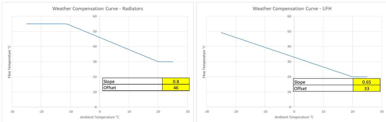
**Figure 35 Sample Weather Compensation settings for Radiators & UFH**
