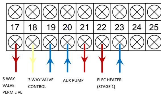
**Figure 32 Installer's Digital Output Connections (AS01 & AS02)**
