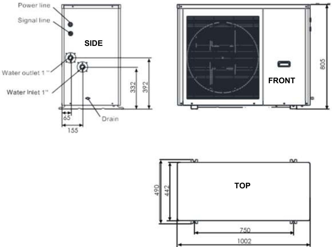
Figure 23 AS01-R32 Casing Dimensions & Heating Connection Locations
