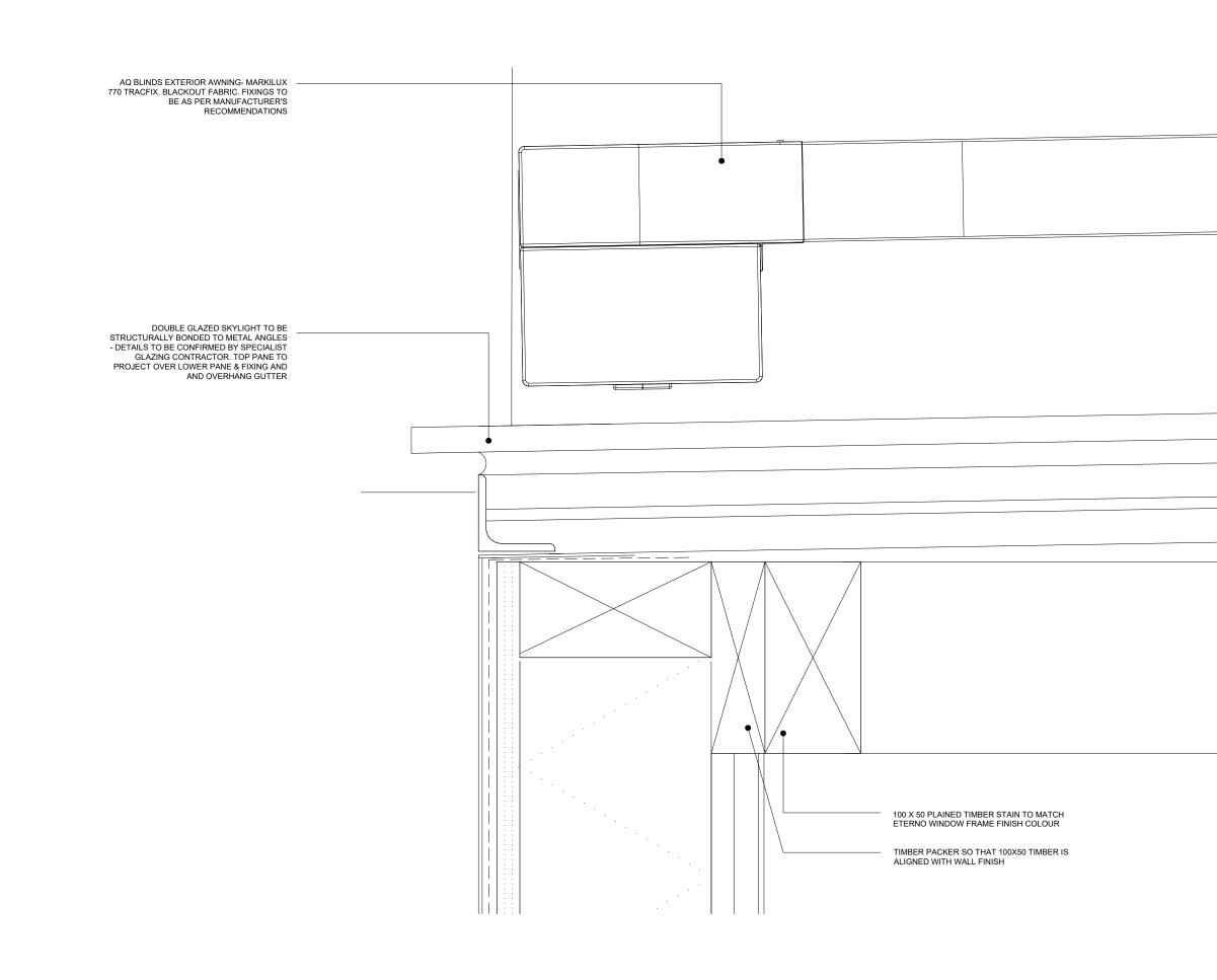
PROPOSED SKYLIGHT DETAIL - LONG SECTION 1:2@A3
