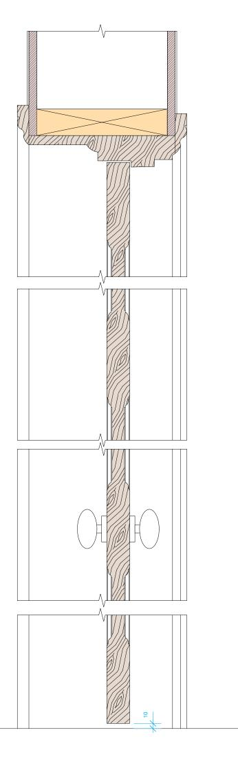
Third Floor Door Head and Threshold Detail S 1:5
