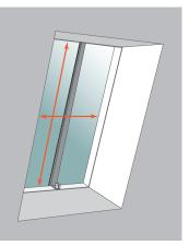
Viewable Area The area of glass that is viewable from inside the room. Please measure the width and length at its closest point to the glass.
