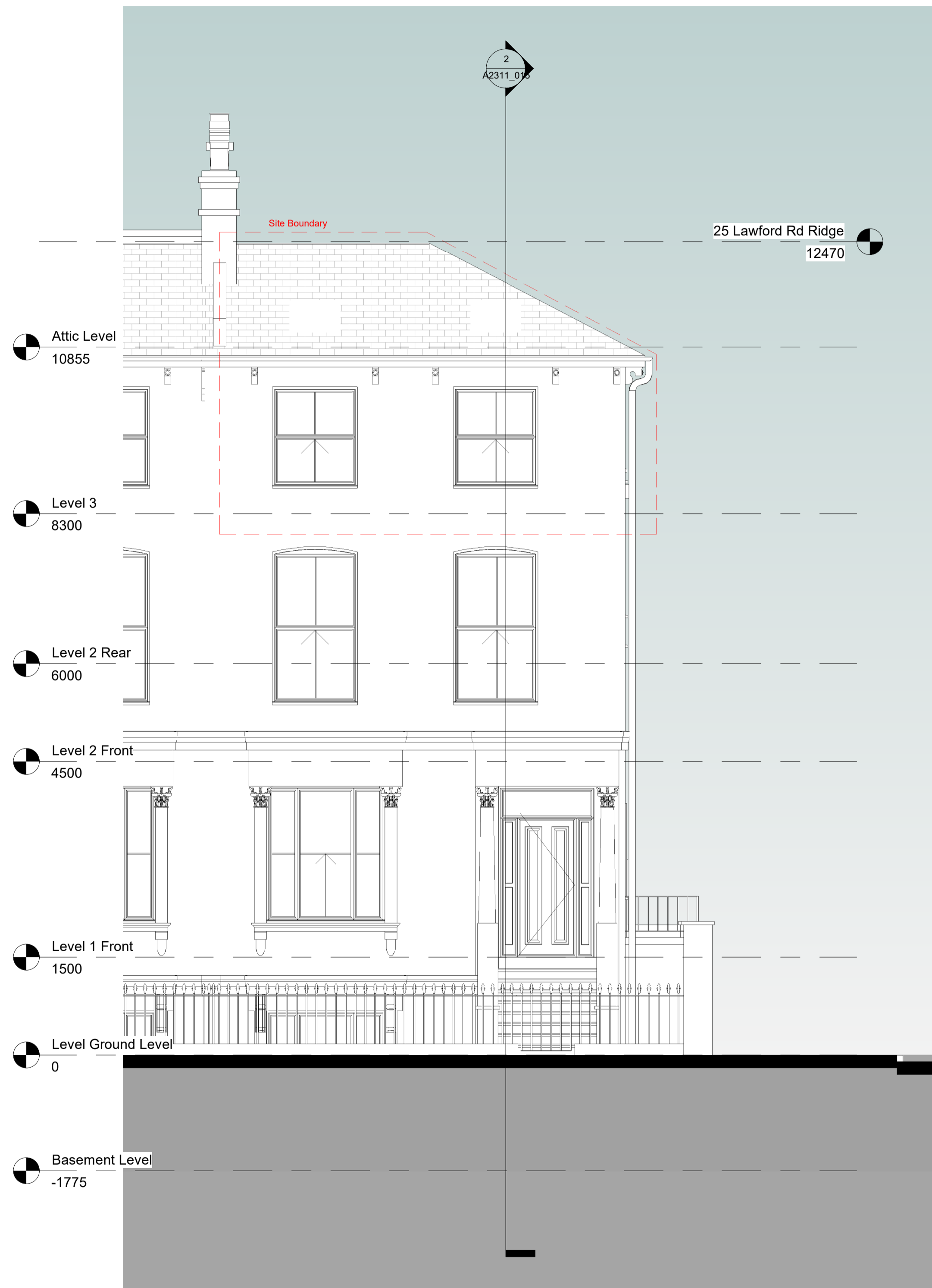
1 Existing South Elevation 1 : 50
