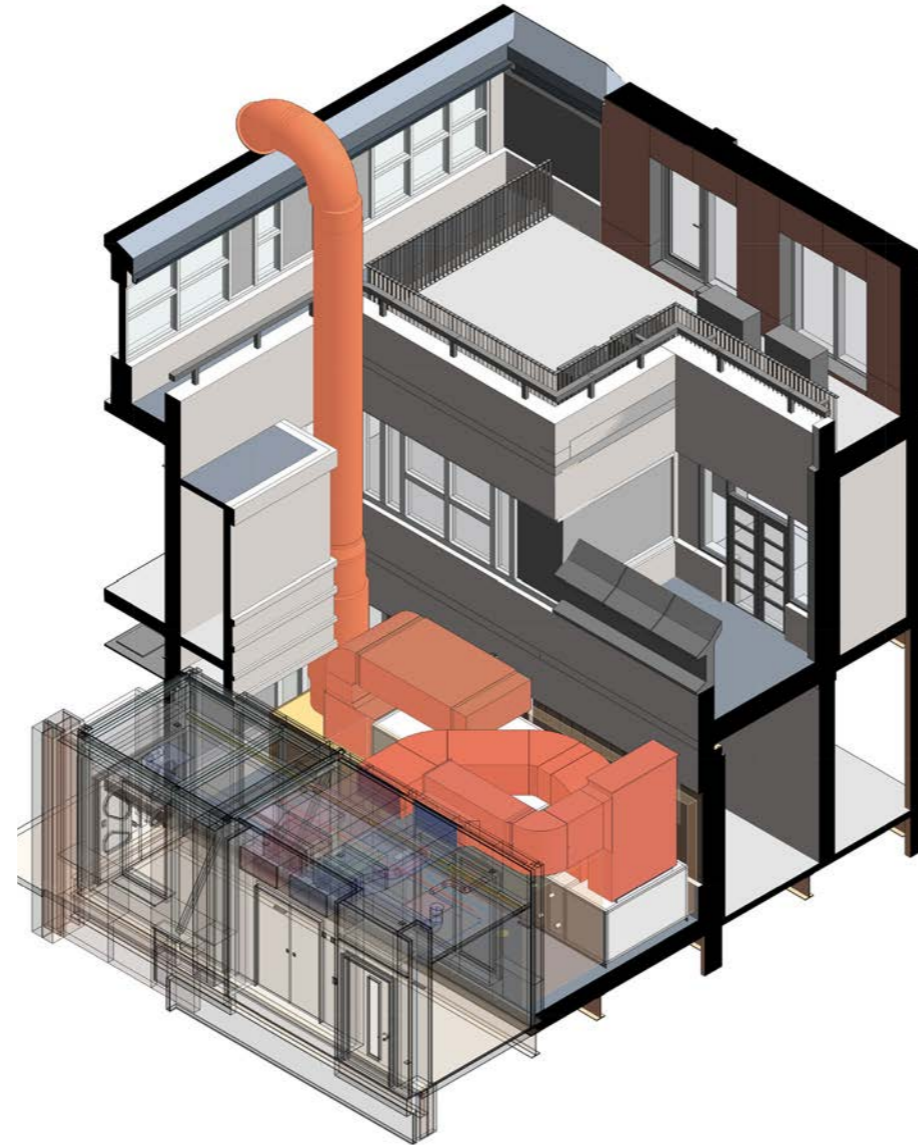
Proposals to re-provide the Cheetah Ward AHU on the Level 4 VCB terrace
