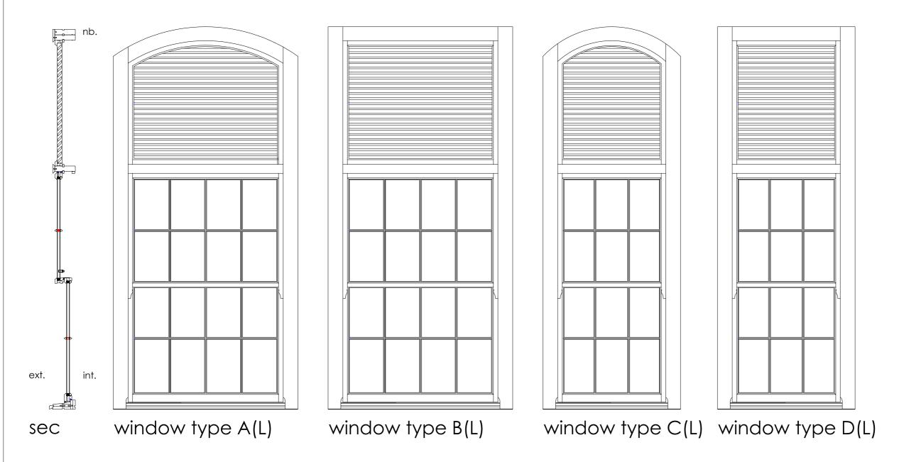
Bereco traditional sliding sash window to achieve 1.2 W/m²K with integrated hardwood louvre to accommodate MVHR extract
